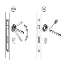
Take out squere rods and use it to strip the steering washer that sits in the middle of the mounting washer
