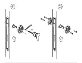
After making markings, please drill the surface of the interior of doors stile in 90 degrees angle. Screw in the mounting washers with the supplied screw and socket
