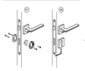
Screw in the mounting washers with the supplied screws. Center the square rod in the lace. Press the outer parts so that it clicks into the base on the upper side of the mounting washers. Screw in and tighten all stop screws
