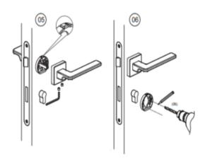
Center the square rod again. Check that the hollowed-out part of the spar is positioned correctly so that it will meet the stop screw in the handles. Press the handles firmly so that it clicks into the heel on the upper side of the mounting washers. Tighten with the allen key all 4 screws. The smaller stop screws must be mounted in the rosettes, while the larger ones must be mounted in the handle itself
